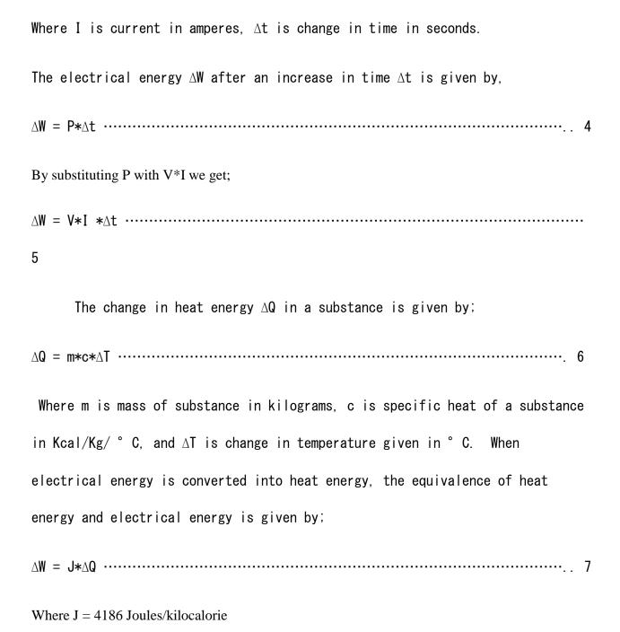
In this experiment a constant current (I) flowed through a resistive heating element and a constant voltage drop V was determined. Temperature is measured as a function of time. The electrical energy which was expected in this element was transformed to heat energy. This heat
